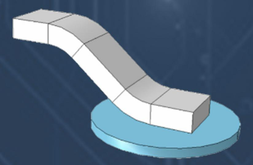
• A user-defined lead is supported. User may generate an arbitrary lead in Abaqus/CAE, then QustomPCB manages the placement along components and the merging or tying of the leads to the board and components
